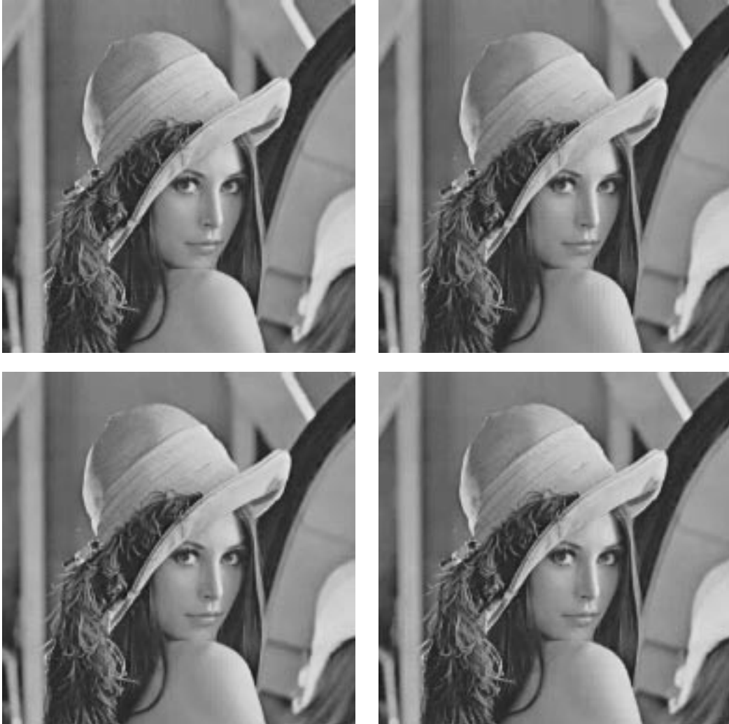
Figure 12: Original and compressed images for Lena. (top left: original, top right: JPEG, bottom left: equal parity, bottom right: biorthogonal)
